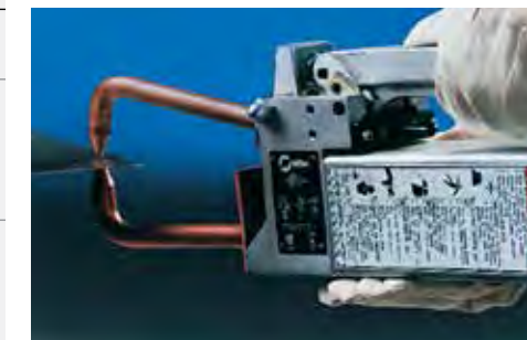
Gyro Bail #041 979 Supports the weight of the welder. Operates with boom and counterweight or from spring-loaded cable. Spot welds in any position.
